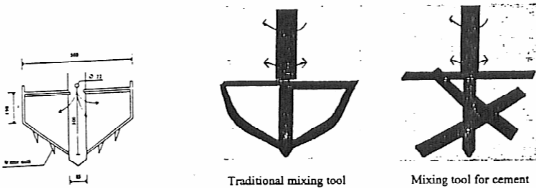
Details of Mixing tools for Lime-Cement columns (Courtesy: Stabilator)
